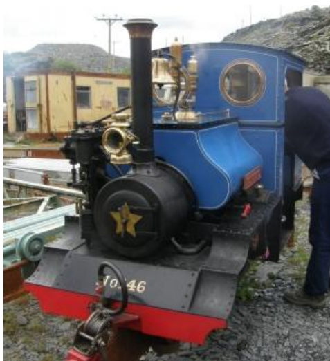
A Monoloco steam engine - part of the Richard Morris Monorail Collection, the loco is really diesel underneath. This locomotive was built in 1997-8)
